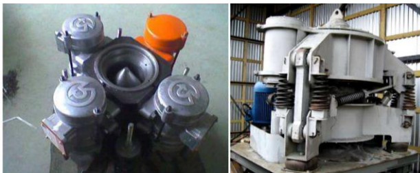
Fig. 7 Vibratory cone crushers with a dual-mass inertial vibrator driving the outer working cone (with a stationary inner cone): WKDC-150 (left – drive by four vibrators) and WKDC-700 (right – drive by one vibrator) manufactured by Mekhanobr Source: [3].
