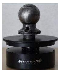
Fig. 9 Preparation of the object on the rotary table
