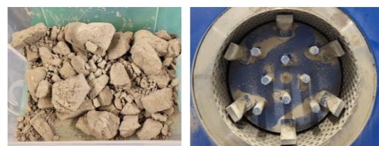
Fig. 1 Fine basalt before crushing and view of the impact crusher chamber
