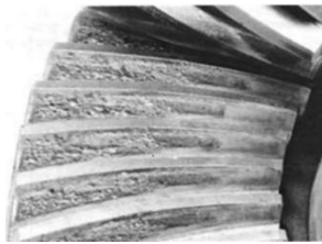
Fig. 3 Destructive (progressive) pitting Source: [30].
