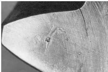
Fig. 4 Fatigue crack Source: [31].
