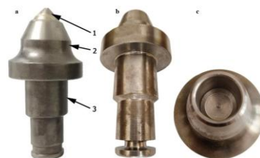
Fig. 1 Construction and basic dimensions of a conical pick: a. construction of the pick, b. pick body, c. a hole in the pick for the tip
