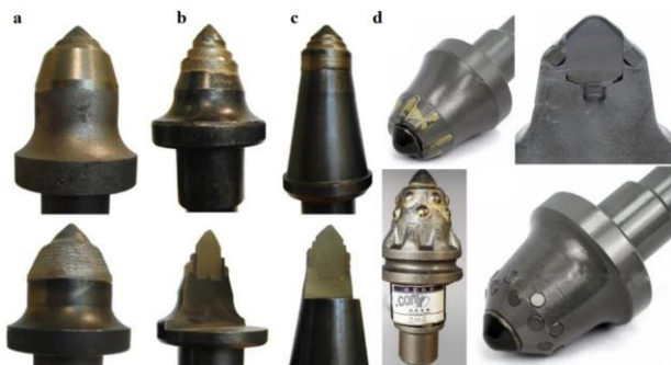
Fig. 3 Ways of increasing the life of picks: a. coated picks, b. pick with a carbide ring, c. pick with two carbide rings, d. pick reinforced with additional carbide tips Source: based on [7].
