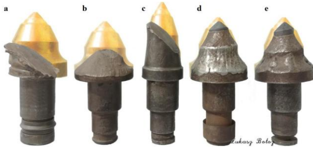
Fig. 2 Examples of conical pick wear after working in a mine: a and c asymmetric, b, d, e symmetric Source: [21].
