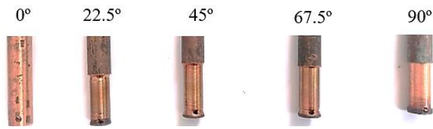
Fig. 2 Electrodes angle with produced by WEDM
