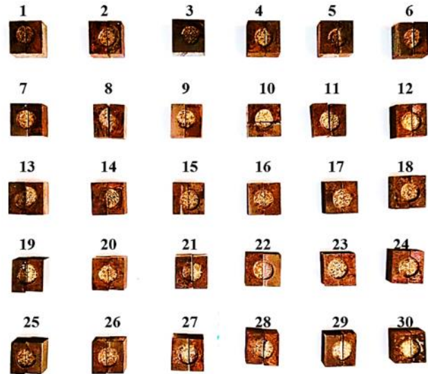
Fig. 3 Alloy steel 30 Workpieces (X210) after machining
