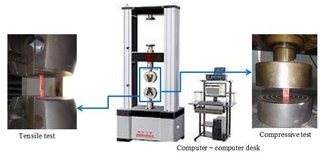
Fig. 5 Mechanical Tests at the WDW-200E Computer Controlled Electronic Universal Testing Machine
