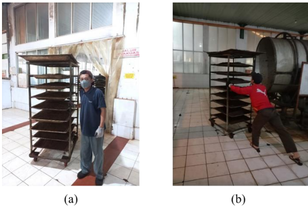
Fig. 1 Current condition of the Trolley Rack: (a) Being pulled, (b) Being pushed
