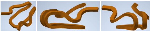
Fig. 9 Pin used for analysing the influence of 3D printing orientation
