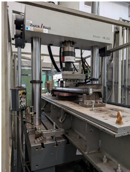
Figure 13. Rail sample 60E2 R350HT in the vertical fatigue strength test.
