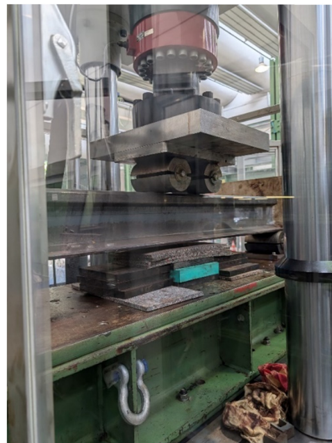
Figure 12. Rail sample 60E2 R350HT in the vertical fatigue strength test.
