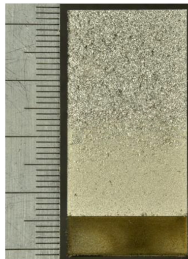
Figure 10. Fracture of sample numbers 4–3 for determining the fatigue crack growth rate.
