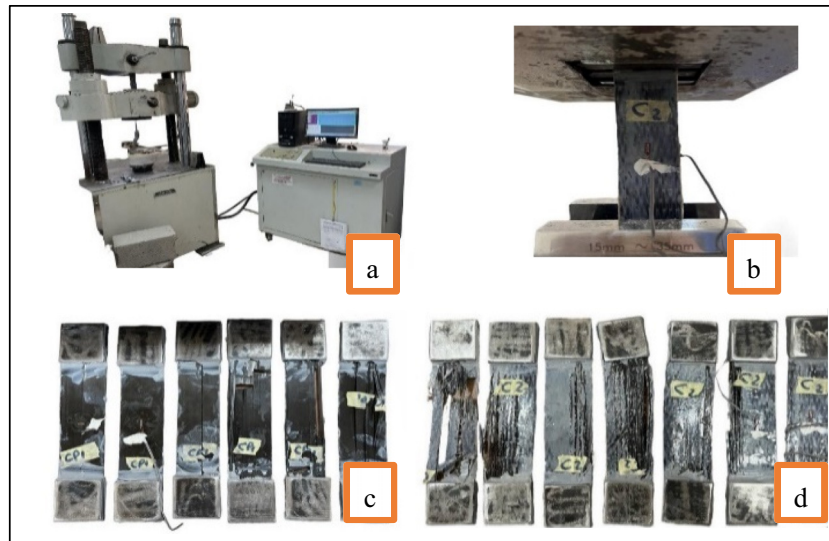
Figure 2. CFRP coupon testing: (a) universal machine test; (b) coupon under testing; (c) laminate CFRP coupons failure; and (d) fabric CFRP coupons failure.
