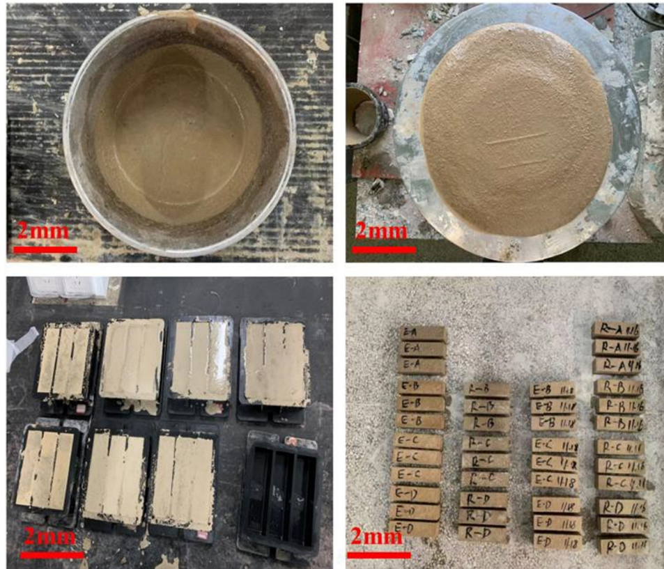
Figure 1. Preparation and curing of EVA PMCSAC mortar specimens.
