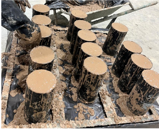
Figure 3. GPC cylindrical specimens during casting.
