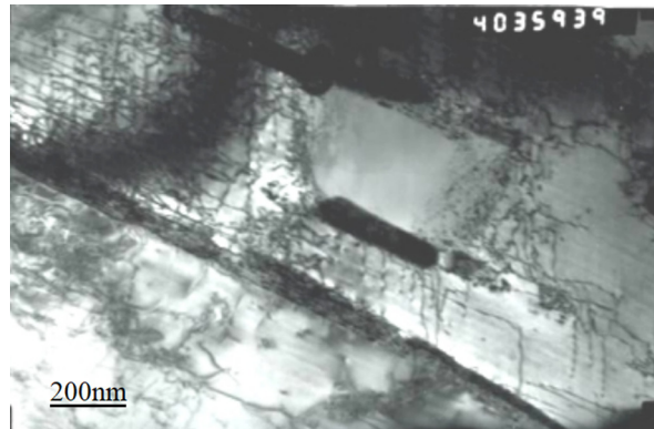
Figure 12. Microstructure of martensitic steel after 90,000 h of operation.
