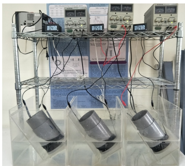
Figure 3. Test setup of rapid chloride migration test.
