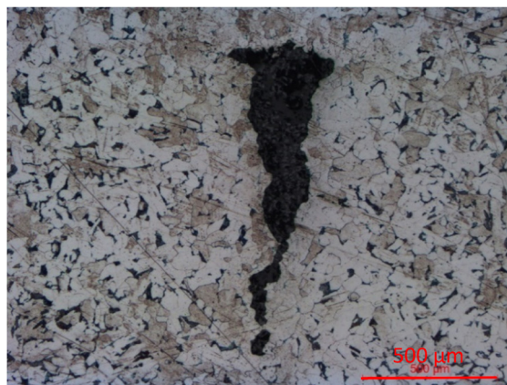
Figure 26. Image of a non-metallic inclusion – low carbon steel (Aachener Hütte), sample No. 3.
