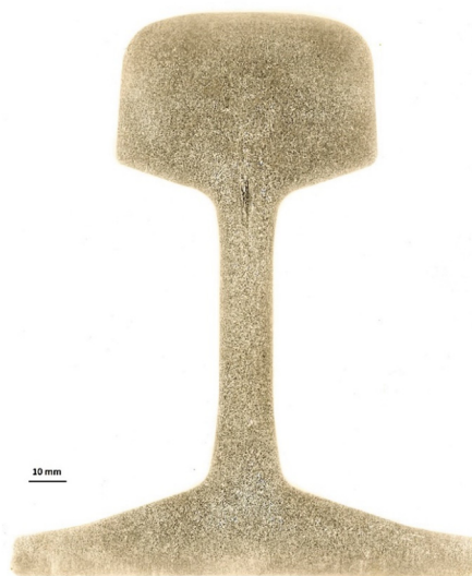
Figure 19. Baumann print, sample no. 6.
