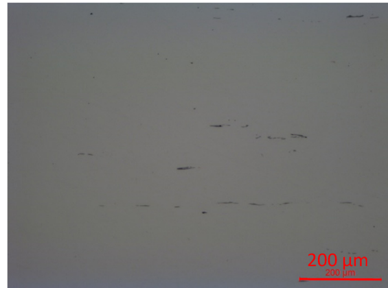
Figure 29. R260 steel with MnS inclusions.
