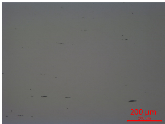
Figure 30. R350HT steel with MnS inclusions.
