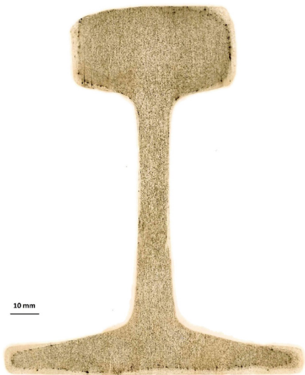
Figure 15. Baumann print, sample no. 2.
