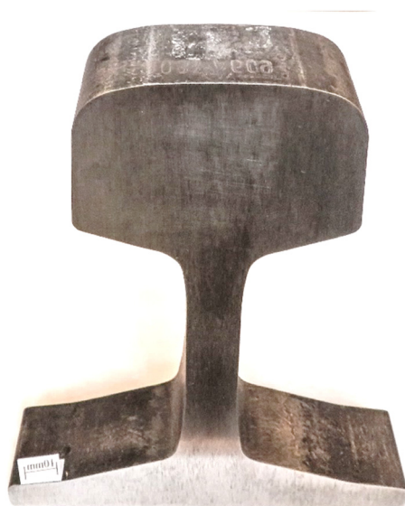
Figure 5. ArcelorMittal Poland S.A. rail in steel grade R260.
