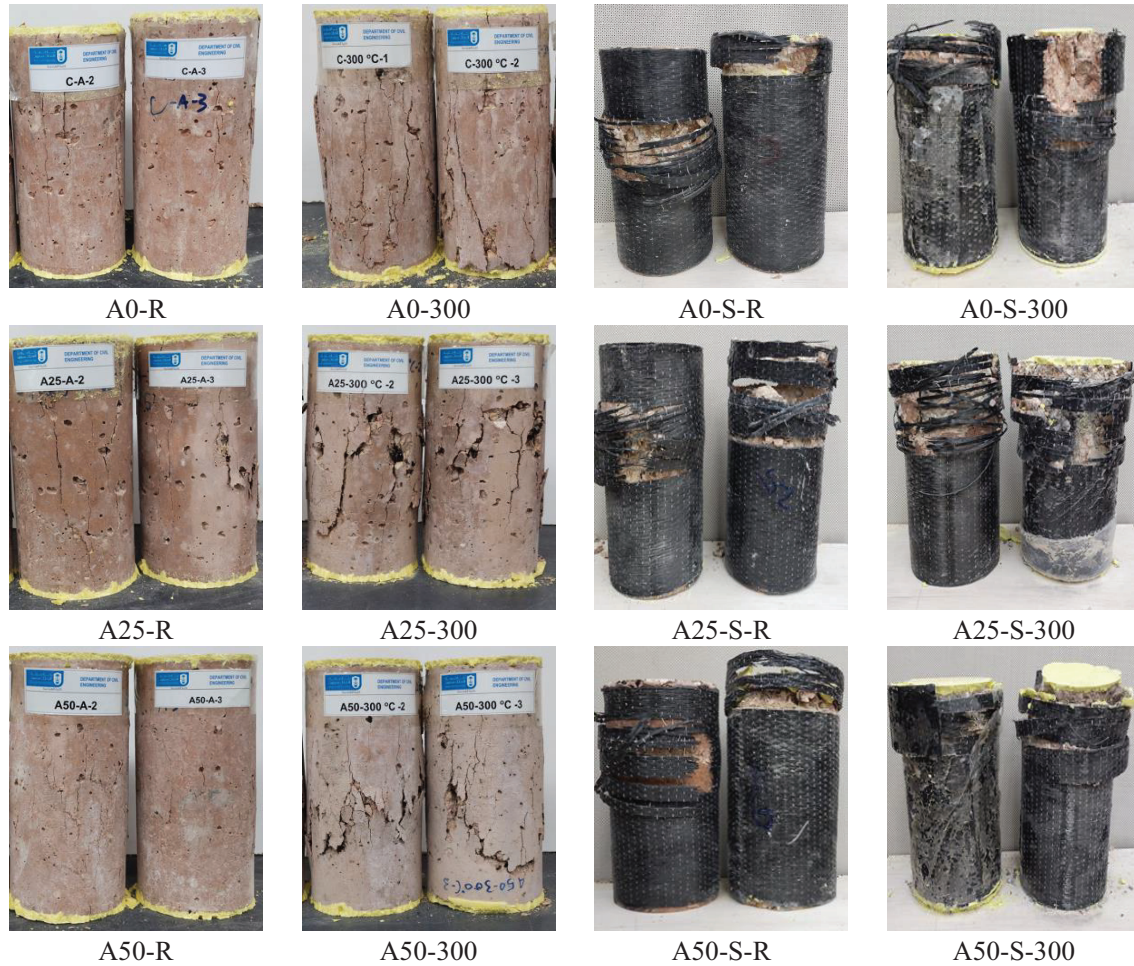
Fig. 8. Failure mode for all specimens
