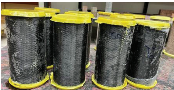
Fig. 5. The specimens strengthened by CFRP sheets
