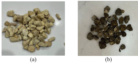
Fig. 3. Samples of the coarse aggregates used in this study. (a) Limestone aggregate. (b) RAP aggregate
