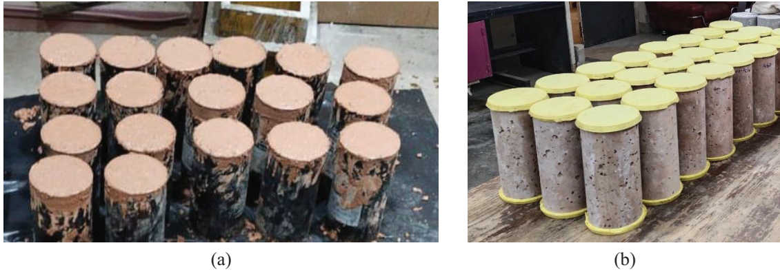
Fig. 4. Specimen preparation. (a) Cylinders during casting. (b) Cylinders ready for testing
