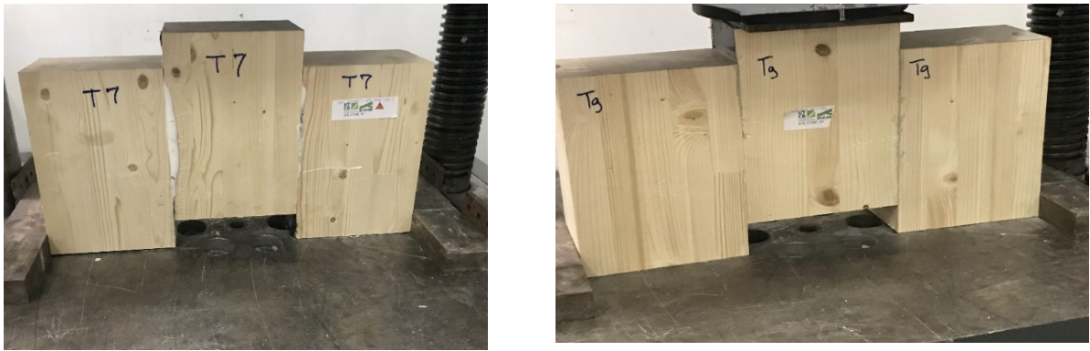
Fig. 2 - Experimental images for shear test
