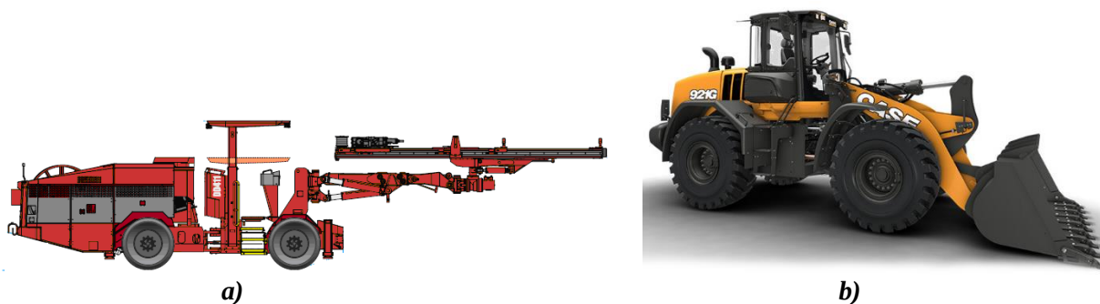
Fig.10. Machines and equipment for the mining technology of extracting lumps rock salt a) SANDVIK DD411 jumbo; b) 921G CASE wheel loader
