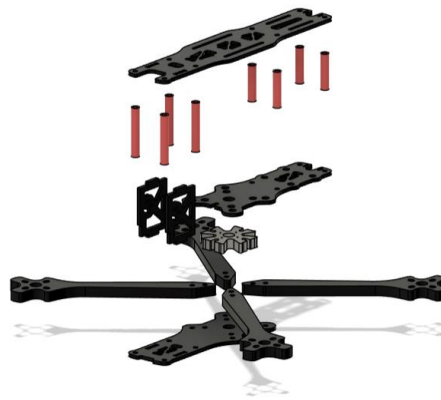
Fig. 1 The view of the construction of the FPV drone's body. Source: authors
