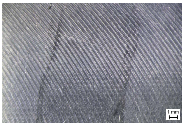
Fig. 8. Darkening of the epoxy resin LH 210 after acetone application
