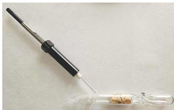
Fig. 3. Extraction of VOCs using a DVB/CAR/PDMS SPME fibre
