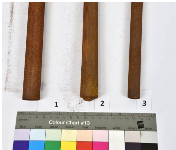
Fig. 4. Appearance of the barrel samples after application of the fourth layer of the cold blackening solution
