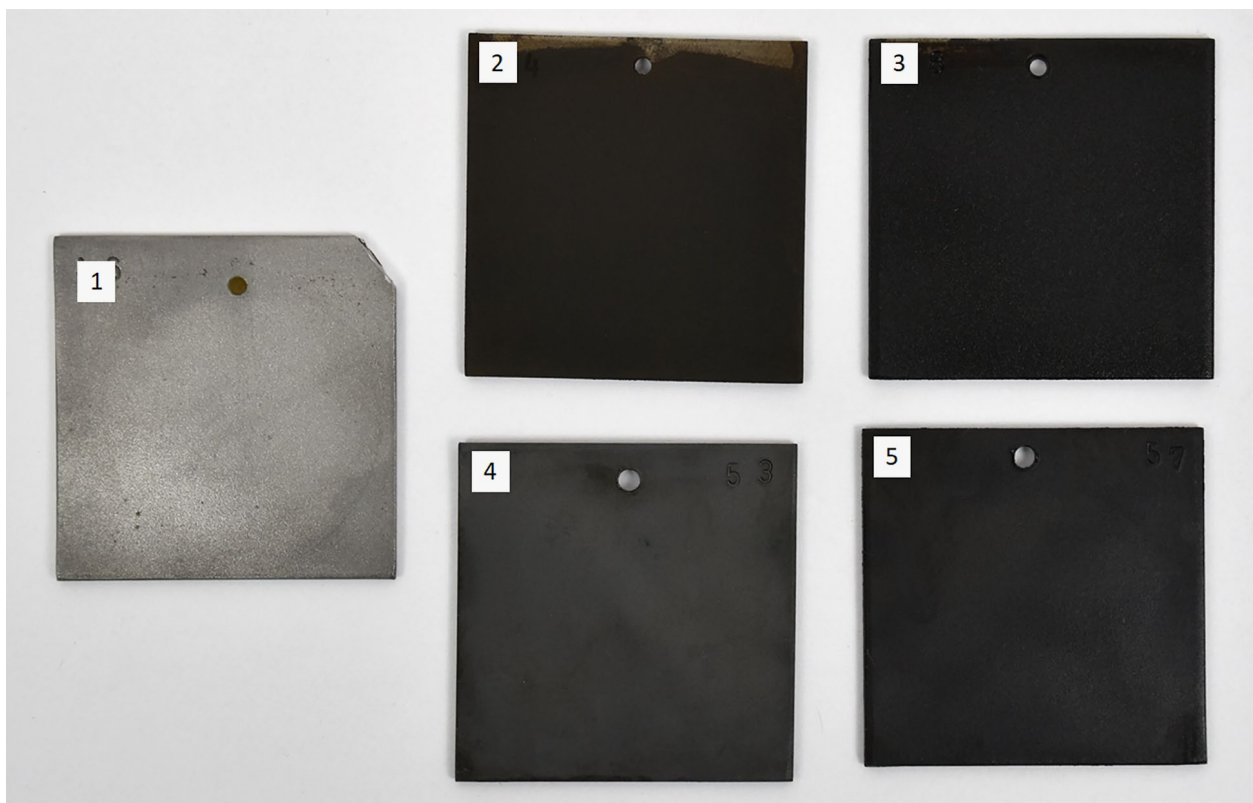
Fig. 8. Appearance of blackened samples (1 – blank, 2 – acid blackening, 3 – acid blackening with preservation, 4 – alkaline blackening, 5 – alkaline blackening with preservation)
