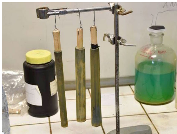
Fig. 3. Appearance of the barrel samples after application of the first layer of the cold blackening solution
