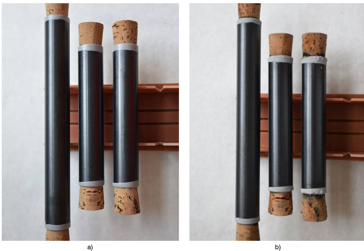
Fig. 7. Samples of alkaline blackening before (a) and after corrosion testing (b)
