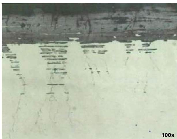
Fig. 9. Light glycidic etched structure revealing inclusion's dissolution at the crack-path interface. A few inclusion at cracks/inclusion-intersections were dissolved by hydroxyl ions
