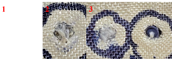
Figure 5. Details of panel front for the impacted zones.
