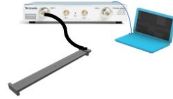
Figure 1: Setup used for measuring the relative complex permittivity and loss tangent of flower leaves
