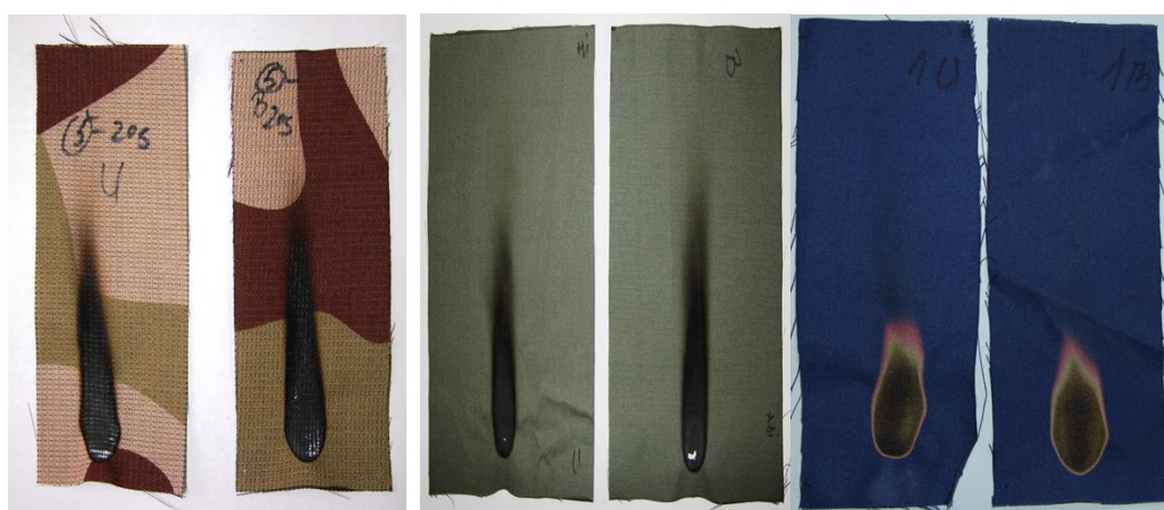
Figure 3: Burning behavior of outer layer materials (M-left, XA-center, Nomex-right)
