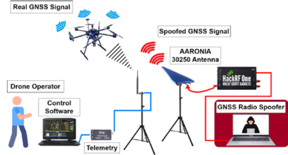
Figure 15: Pixhawk DIY drone –scenario architecture for telemetry control mode
