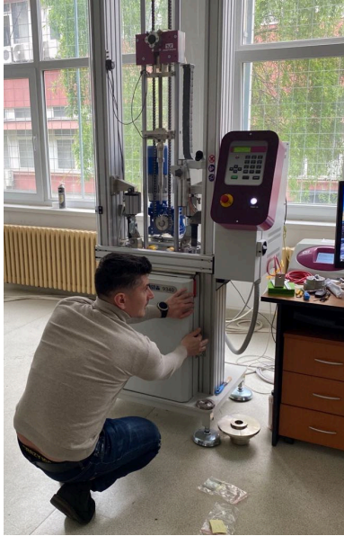
Figure 1: Instrumented drop weight impact tester (CEAST 9300 Series -Instron) during tests
