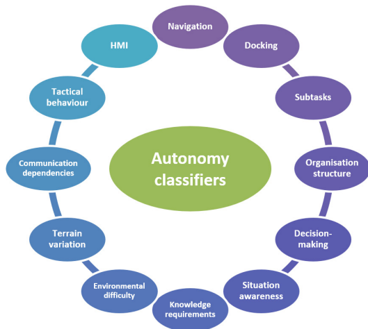
Figure 4: Autonomy classifiers of an A-UGV (adapted from [6])
