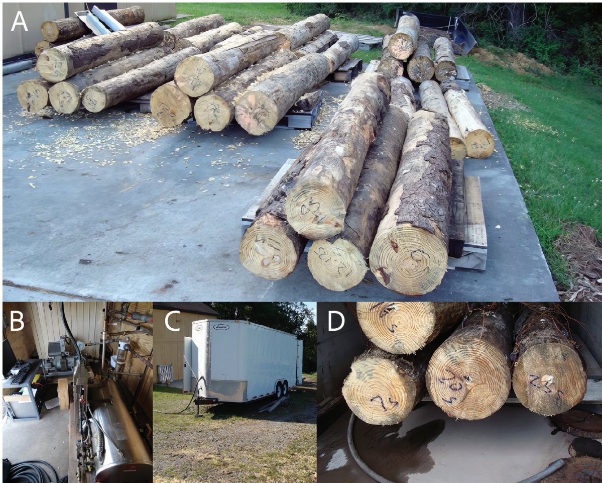
Figure 2: A) Whole yellow pine ( Pinus spp.) logs were debarked at the woodlot and shipped to the research lab at Virginia Tech, where they were cut into 2.3 m lengths, and groups of four were placed on wooden pallets and randomly selected for the various treatments. B-D) The vacuum treatment set-up used in this research was custom-built inside a mobile trailer with a vacuum container, and the steam generator was used as the test chamber with the capacity to treat 4 whole 2.3 m logs at the same time. Temperature sensors were attached to the log at the same time at various sites on the log and inside the chamber.
