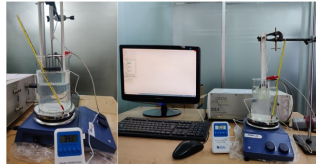
Fig.3: Experimental setup for impedance measurement from different biological samples using a bioimpedance spectrometer while heating on hot water bath.
