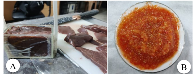
Fig.1: (A) Custom made test cell containing animal tissue sample for measuring impedance while heating on water bath. (B) Mashed tomato sample for impedance measurements at different temperatures.
