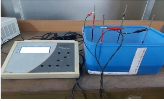
Figure 4: Phantom with electrodes and the instrument for electrical impedance measurement (Maltron Bioscan 920-II) used for the experimental study.
