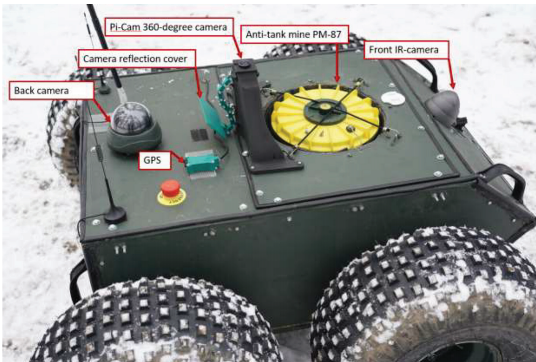
Fig. 2: Laykka platform with mine-module and 360-degree camera module installed on top.
