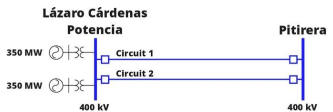
Fig. 7. 400 kV three-phase double circuit
