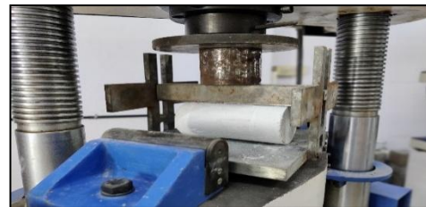
Figure 7. Split tensile strength testing
