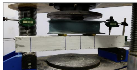
Figure 8. Flexural strength testing
