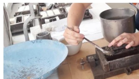
Figure 4. Casting compositions in metal mold
