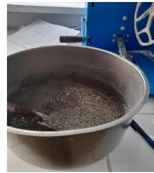
Figure 2. Manual mixing of dry components
