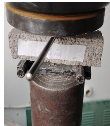
Figure 10. Mortar Sample in Press - Bending Tension Testing
