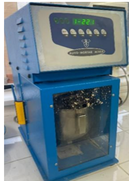
Figure 3. The mechanical mixer used for mixing the mixture
