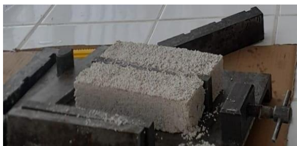
Figure 6. Stripping of specimens from sample P10
