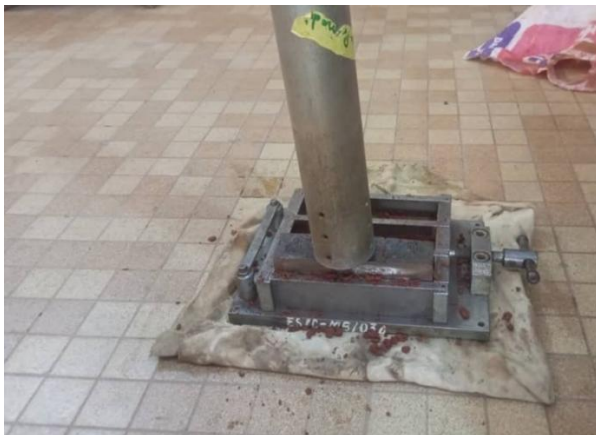
Figure 4. Sample compaction: modified Proctor hammer (A), metal plate (B) 3xmould 4x4x16 cm 3
