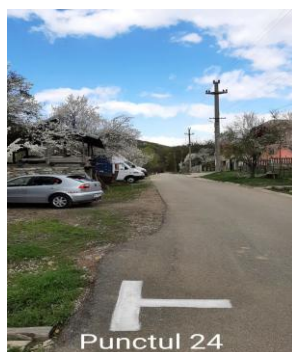
Figure 6. Example of premarked GCP
