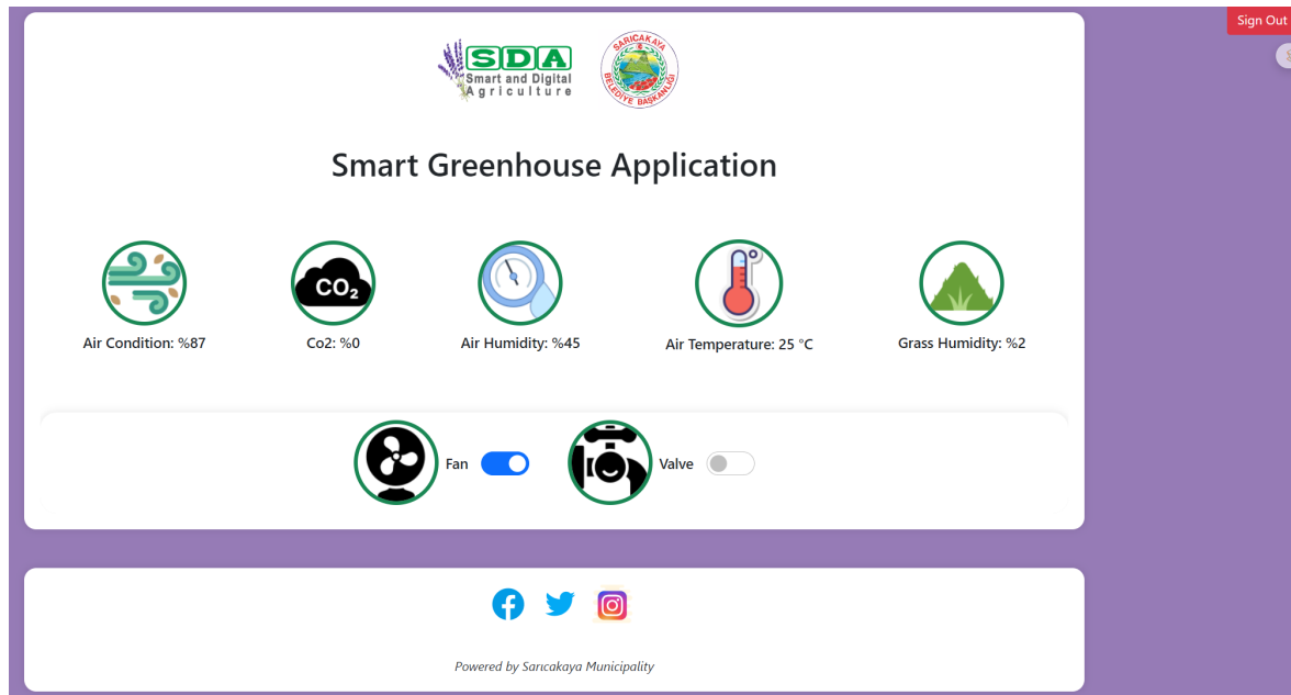
Figure 8: Sensor value-based monitoring interface of the developed Java-based web application.
