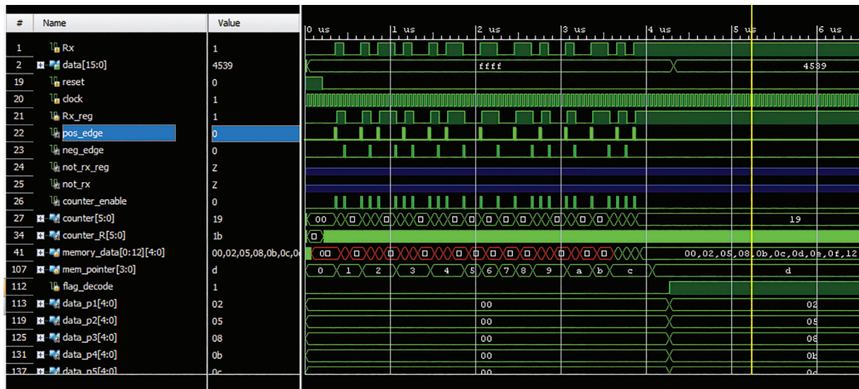
Figure 34: Simulation output of 16-bit DDR ECS receiver module with data input 4539. Double data rate ECS.
