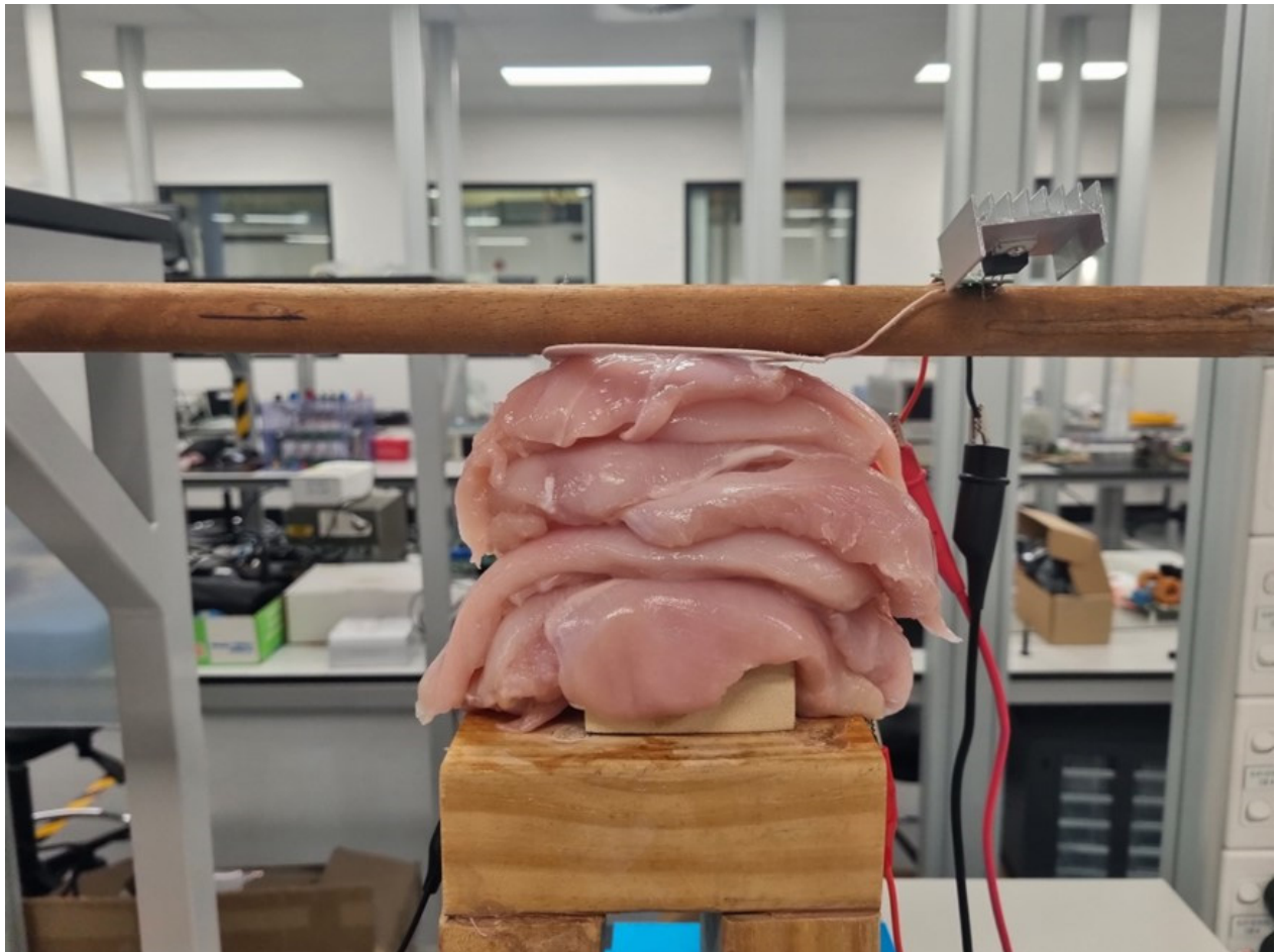
Figure 12: Vertical misalignment testing setup using tissue substitutes.
