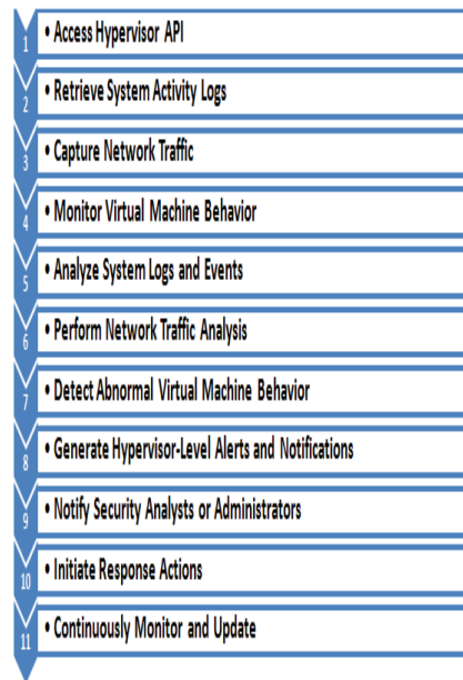
Figure 5. Outline to achieve continuous monitoring at the hypervisor level in the cloud.
