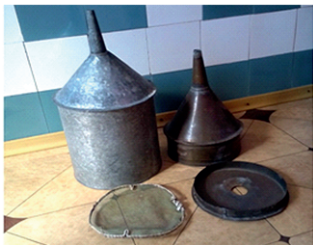
Fig. 1 Berlese-Thülgren extractor in disassembled and working condition.
