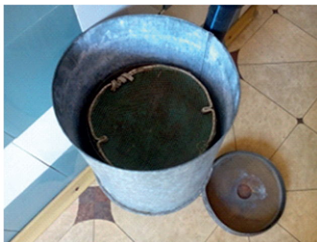
Fig. 1 Berlese-Thülgren extractor in disassembled and working condition.
