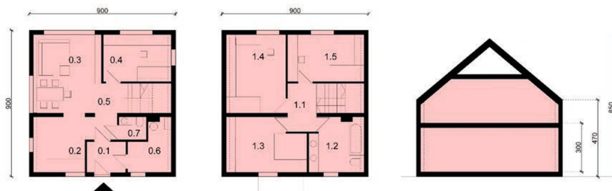
III. 10. Plan and section diagram of the analysed house with 26.0 cm thick external walls. The dashed line shows the outline of the reference building with walls 46.5 cm thick, (by Mika P.)
