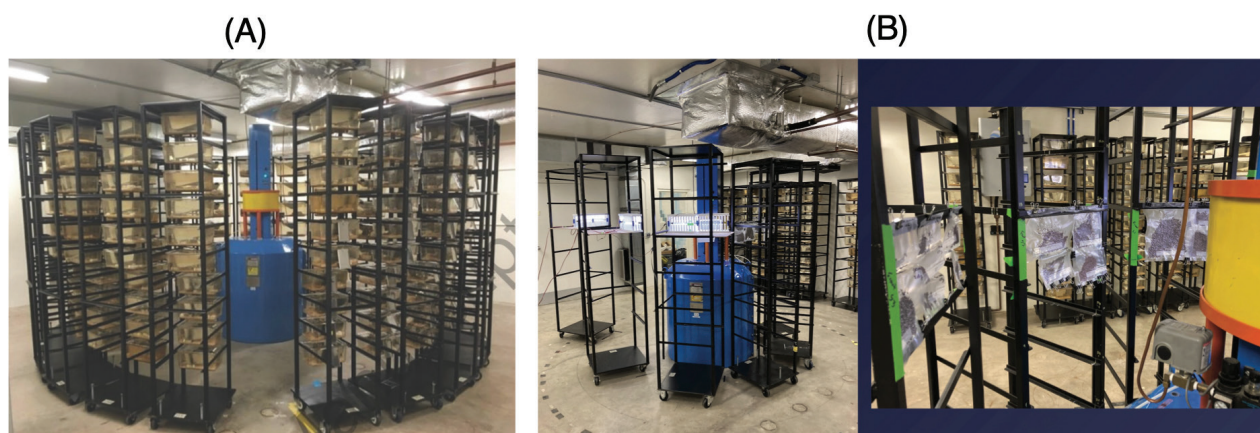
Figure 3. Neutron Radiation Facility at Colorado State University. (A) Rodent radiation experiment setup, showing neutron radiation source in the center. (B) Plant seed radiation setup, illustrating the positioning of seed packets for uniform neutron exposure. Both images are from Dr. Alexander Meyers' 2023 presentation, used with permission.
