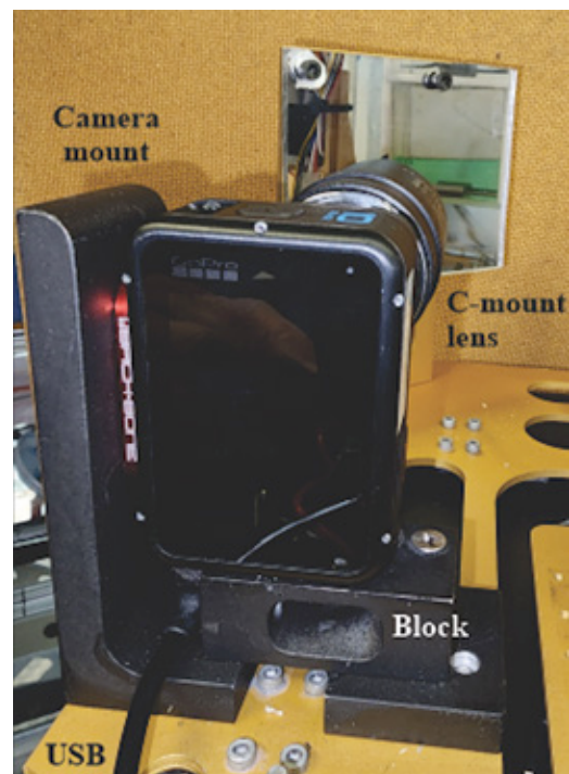
Figure 3. USB connection to the camera to prevent disconnection from vibrations and accelerations. Camera is mounted by two 1/4-20 screws with thread-locking adhesive from the left in this image. The block below the camera is used with a foam block (not visible) to hold the camera battery in place. The cable with right-angle plug has no room to unplug from vibrations or accelerations. An image of the test vessel with green liquid is visible in the mirror.
