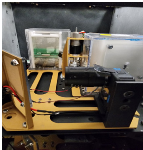
Figure 1. Photograph of one of the four identical cameras mounted in the flight experiment, immediately after the flight. Lens, camera, and mount are all black but note the blue "10" on top of the GoPro Hero-10 camera. Visible red and black wires passing under the mirror on the left and merging into one black cable are the DC power supply to the camera, plugged into the camera USB port that, in this view, is at the bottom of the camera. Black tape on zoom lens prevents boost-phase vibrations from affecting lens settings.
