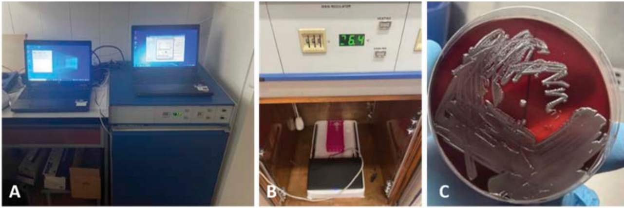
Fig. 2. A- Set of equipment used in the experiment, B- Placement of the exposed sample in the thermostat between the router antennas, C- E. coli cultured on Endoagar
