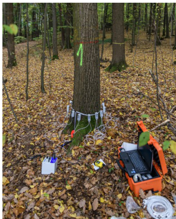
Fig. 1. Measuring equipment with acoustic tomograph ARBOTOM.
