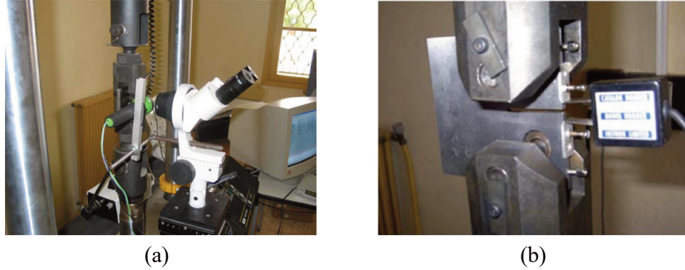
Figure 4. (a) Testing machine; (b) crack opening displacement gauge (CODG).
